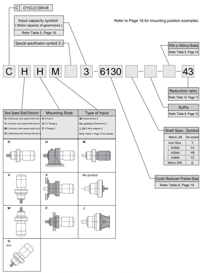
$Note: N: Universal\ Mounting\ Maintenance-free\ is\ for\ Frame\ Size\ up\ to\ 6125(\ Single\ stage\ ),\ 6125DB(\ Double\ stage\ ),\ Galactic (\ Double\ s$
